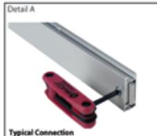
Most horizontal extrusion connections have a patented expandable lock. This lock inserts into the groove of an opposing extrusion. Tightening the lock with the Hex Key Tool expands the lock and creates a strong positive connection.
